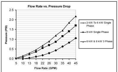
MINIMUM WATER FLOW: 4.4 GPM (265 GPH) MAXIMUM WATER FLOW: 43 GPM (2580 GPH)
